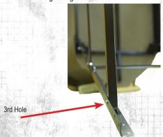
6. Assemble Skis. The skis have a 12" center tube that connects them. Each ski has welded angle on that which determines where it goes. The large welded angle is the front ski. Find the smaller angled (back ski) that shows the angle facing same direction (when laid on the ground) and connect the two with the center splice tube. Do the same to the other ski. Tighten.
