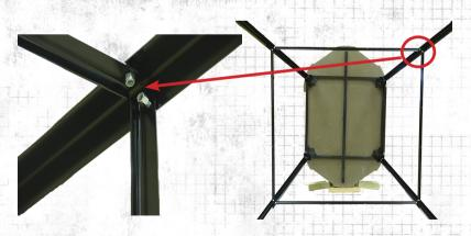
5. Attach (2) 77" Square Tubing bottom support brackets. These go in the opposed direction of the skis, which is vertical in this assembly step. These are attached with 2 ½" L Bolts. Be sure to use the 3rd hole up from the bottom for this bracket. Snug not tighten finish.
