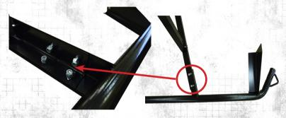
8. Attach 3rd 77" square tubing ladder bottom support bracket to the front skis. This attaches to the inside of the wide angle on top of the front ski.
